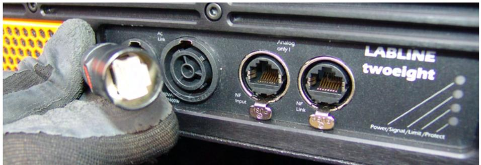
*RJ45-connections are no longer exotic any more. Replacement for a forgotten cable can be purchased in the next computer store. That's not so easily done with an XLR-Cable.*
