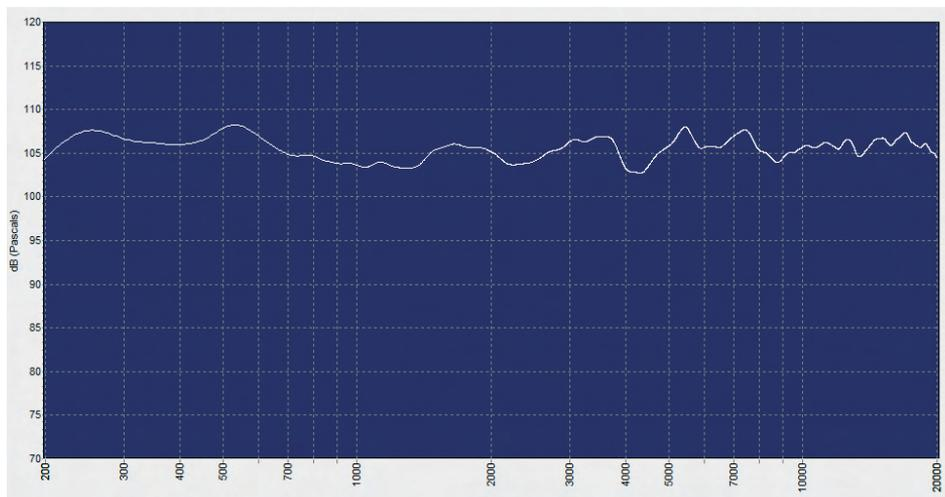
Given that this frequency response measurement was done with the depicted open-air-setup with non-vanishing influence of wind and not in the lab, terms like "ruler flat" are not completely pulled out of thin air. The precision of reproduction is reflected in the visible linearity here.
