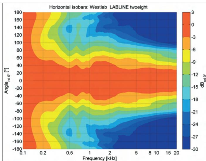
The isobaric view shows the effectiveness of the different measures taken in order to control the horizontal coverage which stays in a range of around 100° relatively independent of frequency.
