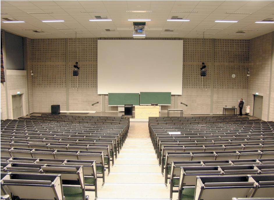
**Room Sorbonne: Acoustical treatment visible on walls and ceiling, but it also comes out clear how compact the sound system is.**
